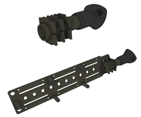
Attach the camera plate to the top plate by pushing the two spacer bolts though the holes in the top plate. They sit tight and you might need a bit of force to push them in.
