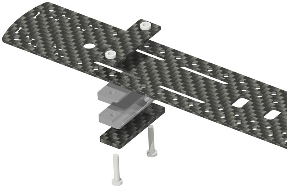
Take care, that the openings on both wing mounts point to the back.
