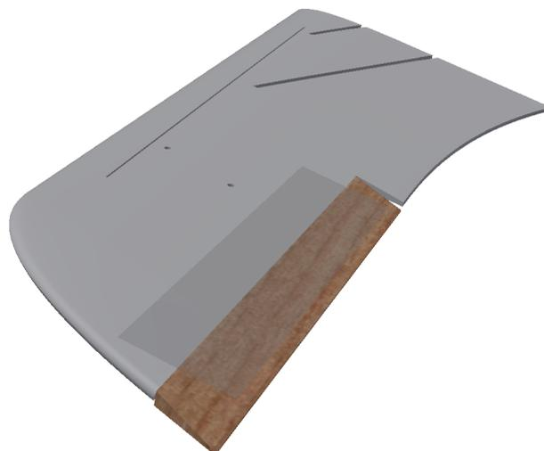
Fold the elevon to the other side so that it lays on the bottom side of the wing. You should see a bit of bent tape between the wing and the elevon. Make sure the edge of the rudder is aligned to the edge of the wing.
